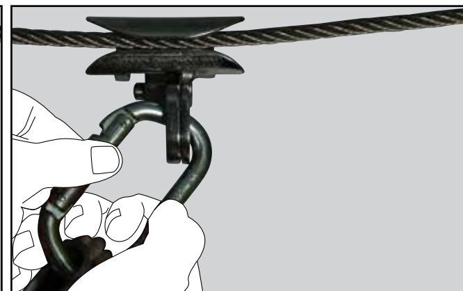
Ensure the karabiner is connected and the screw gate is secured correctly in the closed position.
