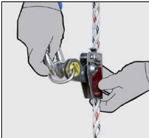
i. (cont) Ensure the casualty's rope is correctly positioned inside the Rescue Rope Grab. Close the Rescue Rope Grab.
