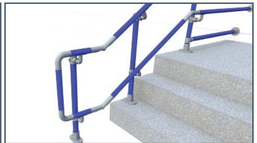
F) EXTENSIONS: Stairs: Handrails should extend the width of one stair tread and then level out for 300mm
