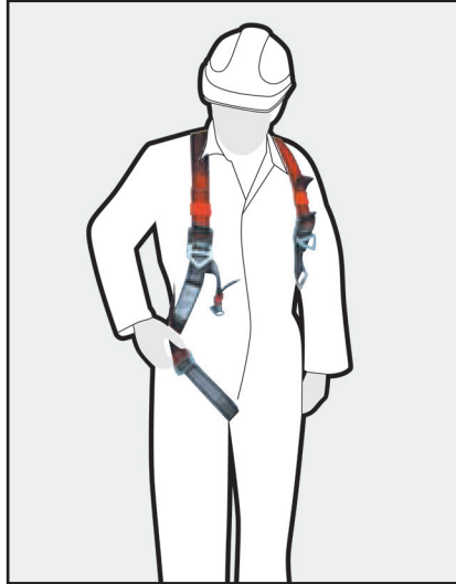
h. Adjust the tension by pulling or releasing the slack end of the strap.
