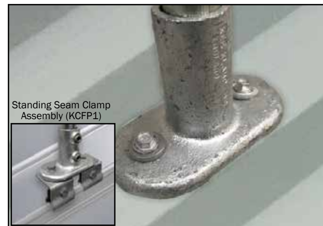
K. Carefully cut 6No. 120mm lengths of sealing strip. Place the Sealing Strip between the 6No. Standard Rail Flange fittings and the roof structure. Use Self Drilling Screws (SDS55X550) to attach the screen onto the roofing sheet. NB If attaching to standing seam roof use KCFP1 clamps to connect to the standing seam and bolt the 62-5 fitting to the KCFP1 clamp as shown in the diagram.
