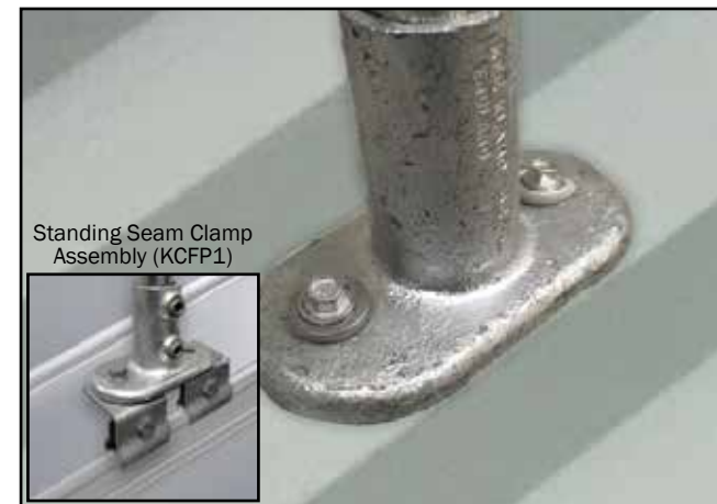
L. Carefully cut 2No. 120mm lengths of sealing strip. Place the Sealing Strip between the 2No. Standard Rail Flange fittings and the roof structure. Use Self Drilling Screws (SDS55X550) to attach the screen onto the roofing sheet. NB If attaching to standing seam roof use KCFP1 clamps to connect to the standing seam and bolt the 62-5 fitting to the KCFP1 clamp as shown in the diagram.
